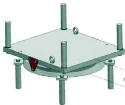
PG8000 - Guided POT Bearing - 8000 kN Maximum Vertical Load : 8000 kN (ULS) Maximum Horizontal Load : 10% Vmax Rotation : 0,01 rad (ULS)
